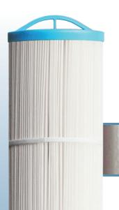
The Green Filtration Series are electropositively charged dual gradient double pleated filtration solutions that successfully remove contaminants from 1 to 0.2 microns, featuring ENPRESS NanoAl<sup>TM</sup> media. The filters are designed with a larger 20 micron pre-filtration layer externally and the charged media internally, extending filtration level contamination and service life, while achieving high flow and low pressure drop.
