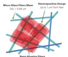
Mean Diameter: 2 nm | Mean Length: 200-300 nm
